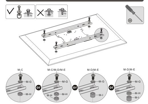
**Note:** Choose the appropriate screws, washers and spacers (if necessary) according to the type of screen. Screw the VESA Plate onto the TV.
