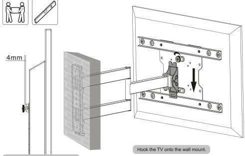
Loosen the upper flat nut leaving a 4mm space to VESA plate.
