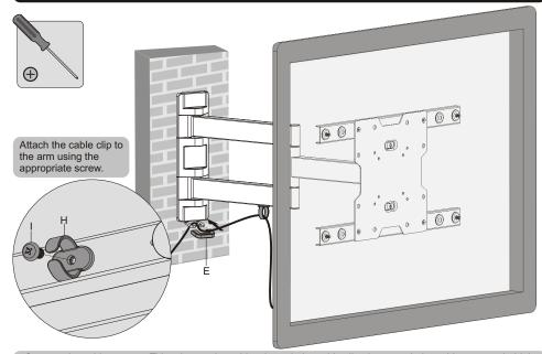
Connect the cables to your TV and route the cables through the cable clip, then attach the cable cover to hold the cable in place.
