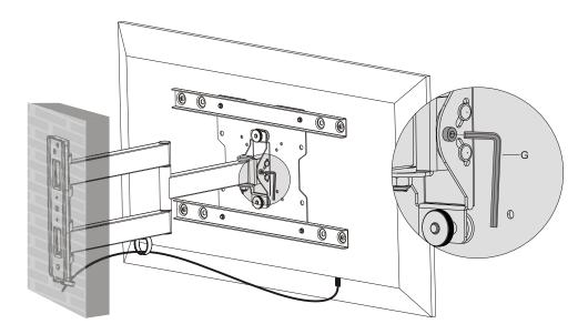
According to the different weight of the display, it is necessary to slightly loosen or tighten the adjustment screw using the supplied Allen key.
