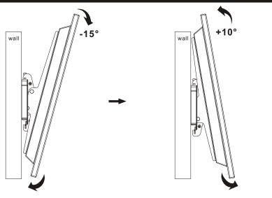
Push or pull from the top or bottom of the display to obtain the desired angle.
