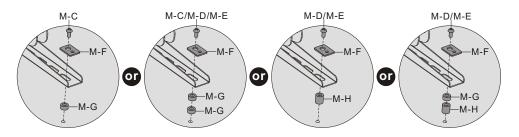
Note: Choose the appropriate screws, washers and spacers (if necessary) according to the type of screen.
