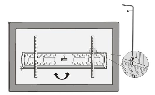
You can slightly adjust to get level for the display by tightening or loosening screws using a 5mm Allen key.
