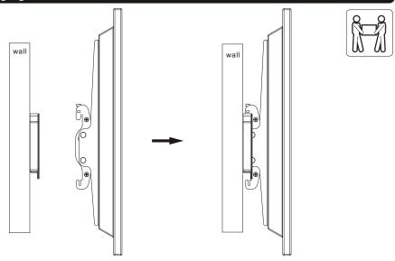
Hook the TV over the top of the wall plate. **Important:** Make sure the TV is correctly hooked before releasing the TV.
